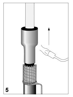
Place the stress control tubing (black) over the core and position it so that it is level with the oversheath cut. Shrink the tubing down starting at the bottom and working towards the core end.
