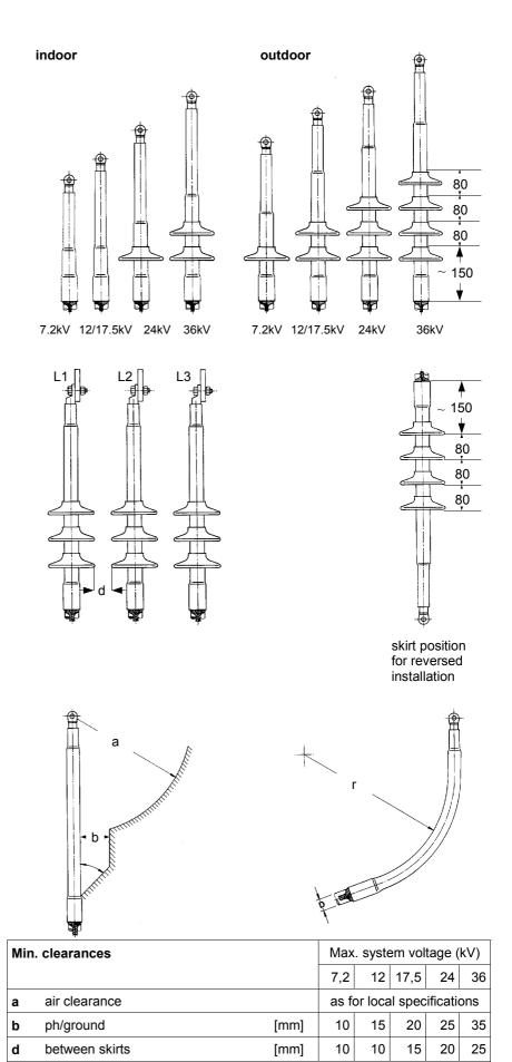
min. bending radius = 15xD, before bending heat cable up to approx. 70°C
