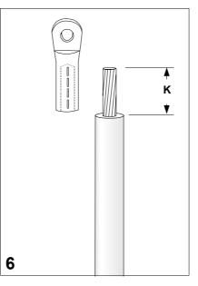
Cut back the insulation according to dimension **K** = depth of cable lug barrel hole + 5 mm. Install the cable lug.
