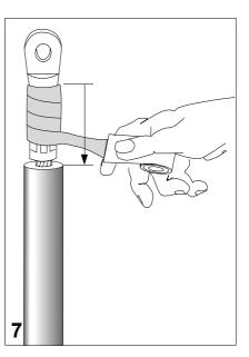
Wrap the red sealant tape around the barrel of the cable lug. Stretch the tape to half of its width and
