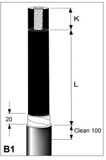
Cut the cable to the required length. Remove the oversheath to the dimension L + K (Table 2). Clean and degrease the end of the oversheath for about 100 mm. Remove the metal tape shield to within 20 mm of the oversheath cut.
