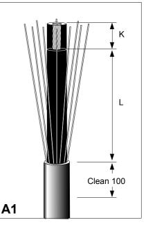
Cut the cable to the required length. Remove the oversheath to the dimension L + K (Table 1). Clean and degrease the end of the oversheath for about 100 mm.
